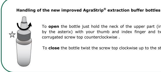
To **open** the bottle just hold the neck of the upper part (indicated by the asterix) with your thumb and index finger and twist the corrugated screw top counterclockwise .
