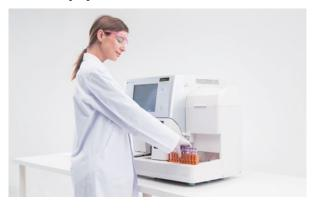
Celltac G's fully-automated random access walk away loading system enables up to 90 tests per hour by just continuously inserting the color-coded racks on the system.
