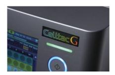
Celltac G status indicator is located in the front panel and clearly illustrates different operating status of the analyzer. For example, the operator can quickly recognize the need for reagent replacement by just looking at the status indicator turning red.
