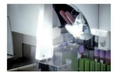
Each tube is picked up one by one from color-coded racks and gently mixed with built-in complete tube inversion mixing arm. Our auto-loading system contributes to faster test report to clinical decision makers and enhances workflow efficiency.
